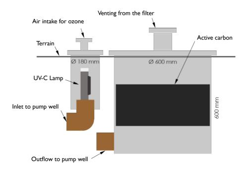
In the hydrogen sulfide filter under ground, the HS Purifier is placed so the UV-C produced ozone gets access to the pump well and is supplied to the well using the HS Purifier's ventilator.
